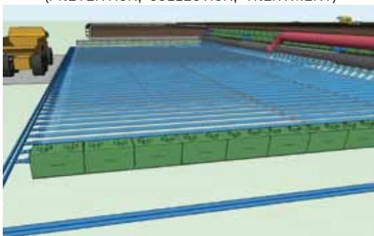
UPGRADED BIOFILTERS (TREATMENT)
